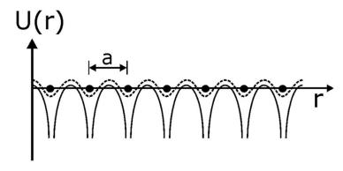
Metals and alloys are crystalline in nature. When the electron move into the periodic ion core, it enters into the periodic potential i.e. potential is minimum at the positive ion sites and maximum between the two ions.
