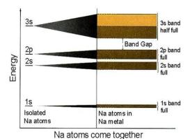
In an isolated atom the electrons are tightly bound and have discrete sharp energy levels. When two identical atoms are brought closure the outermost orbit of these atoms overlaps and interacts. Then the energy levels corresponding to those atoms are split into two. If more atoms are brought together more levels are formed and for a solid of N atoms each of energy levels of an atom split into N levels of
