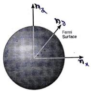
The number of states with energy less than  $E_f$  is equal to the number of states that lie within a sphere of radius  $|n_f|$  in a region of K-space where  $n_x$ ,  $n_y$  and  $n_z$  are positive.
