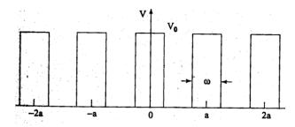
Within the wall the electron has potential energy
